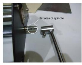
Attach the handle to the spindle of the printing press body. Slide the handle onto the spindle of the bottom roller. Using the allen key tighten the screw of the handle and ensure that flat area of this spindle lines up with the screw for a secure grip.
